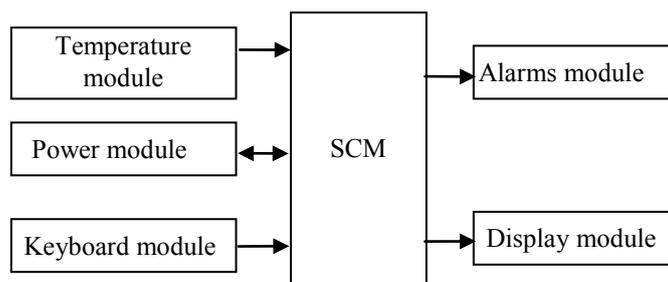
Figure 2: Whole structure of thermometer.
